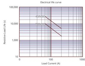
Remark: Rated electrical life number is based on resistive load. Test under switch on/off. Switch on for 0.6s and off for 5.4s.
