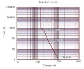
Note: The above data is measured under the conditions of ambient temperature 85°C and the sectional area of conductor wire ≥50mm<sup>2</sup>. The data is for reference only, do not use it to select fuse directly.
