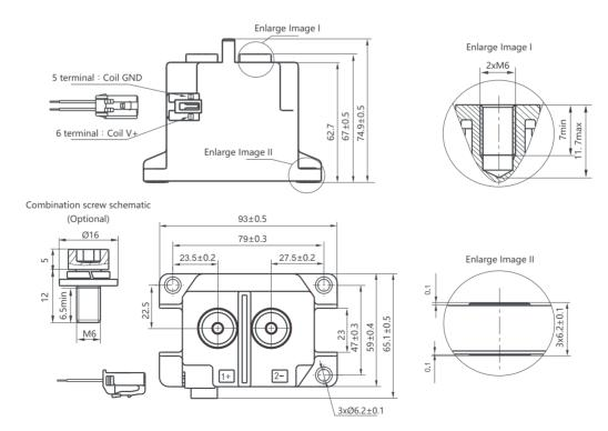
Note: The external dimension of part of the product is not marked with tolerance. When the external dimension is  $\leq 10$ mm, the tolerance is  $\pm 0.3$ mm; When the external dimensions are between ( $10\sim50$ ) mm tolerance is  $\pm 0.5$ mm; When the external dimension is > 50mm, the tolerance is  $\pm 0.8$ mm.
